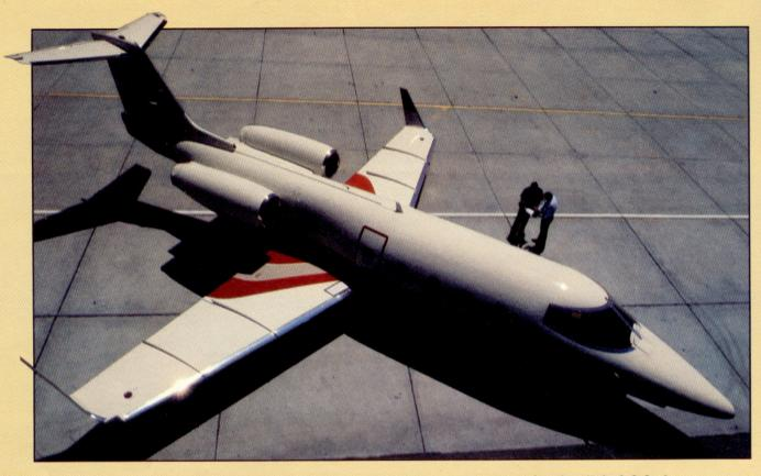
Smooth lines and a new wing give the Lear its speed. At 51,000 feet and .79 Mach, the wing and winglet shock waves buzz as they collide.
